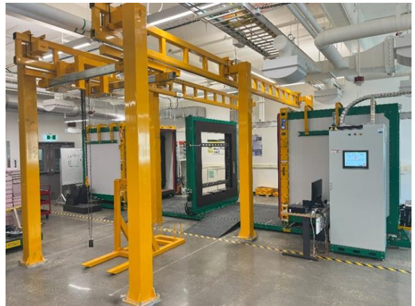
The environmental chamber with the thermal testing frame (green frame)
