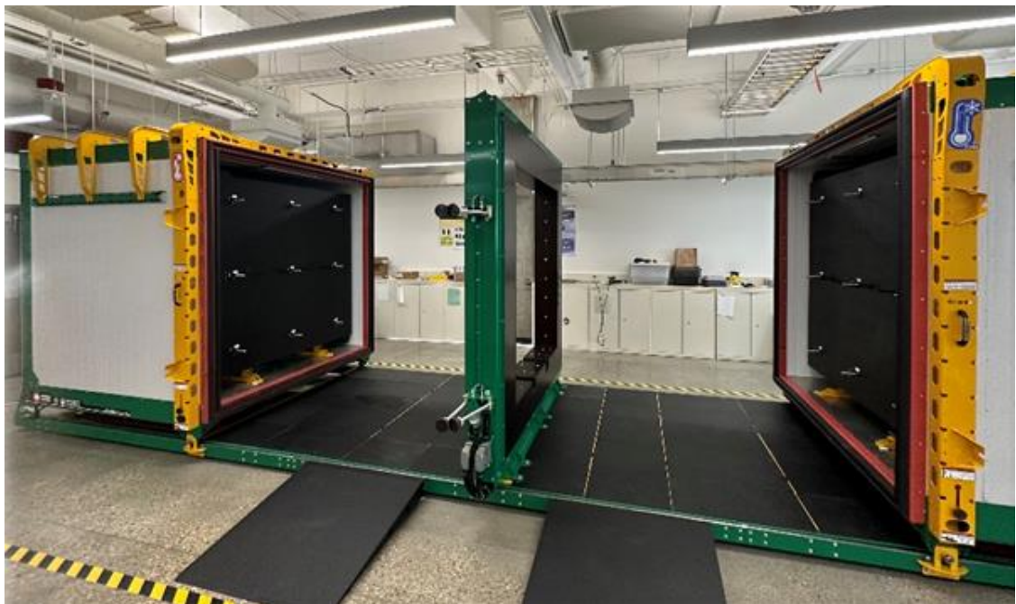
The environmental chamber with the thermal testing frame (green frame)
